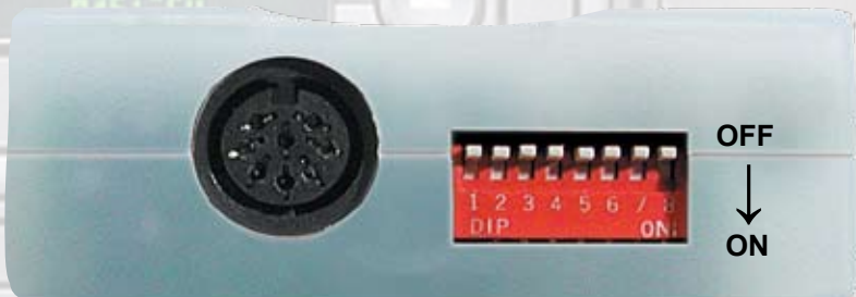
Fig.1 Side view of Interface with dip switches
